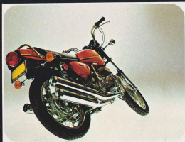
As you can see, the upswept muffler design not only looks great, it also increases bank angle quite a bit.
