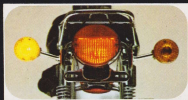
The amperage of the battery has been doubled to carry the extra electrical load of this bigger, safer tail light.
