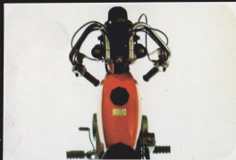
Handlebars fold all the way down for easy transporting in car, boat or plane.
