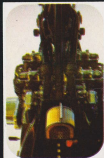
With the gas tank removed, all parts are serviceable with engine still in frame (except crankshaft and transmission).
